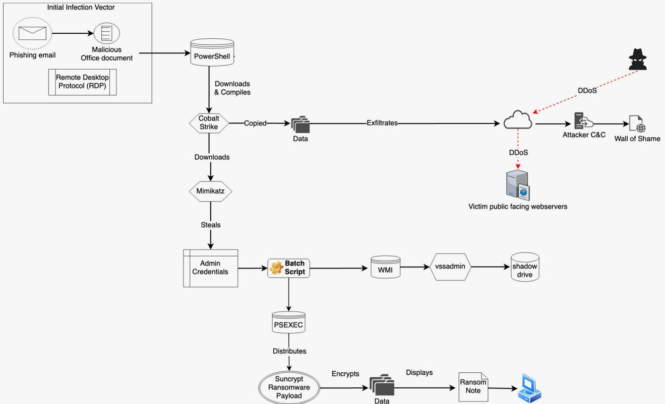
Figure 19: SunCrypt Gang attack chain
