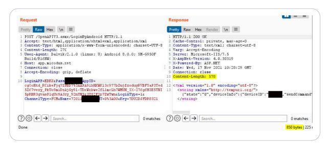
The reply packet of a successful login included a significant volume of information about the device itself, hence the 850 bytes, versus the failed login at 373 bytes. By generating "random" Name fields, testing the default 123456 password, and measuring the size of the replies, we determined the existence of the default password.
