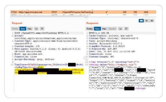
When the user exits the Android application and later returns, this key is not saved anywhere nor is it used again. Instead, a hardcoded key working for all users is stored in the Android app: 7DU2DJFDR8321
