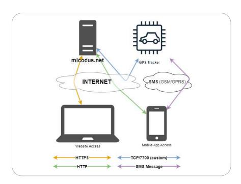
All services appear to be hosted by a single web server (www.micodus.net/47.254.77.28). It provides a website via HTTPS port 443, an API server to support mobile apps via HTTP port 80 (app.micodus.net/47.254.77.28) and a GPS tracker custom protocol server running on port 7700 (d.micodus.net/47.254.77.28).
