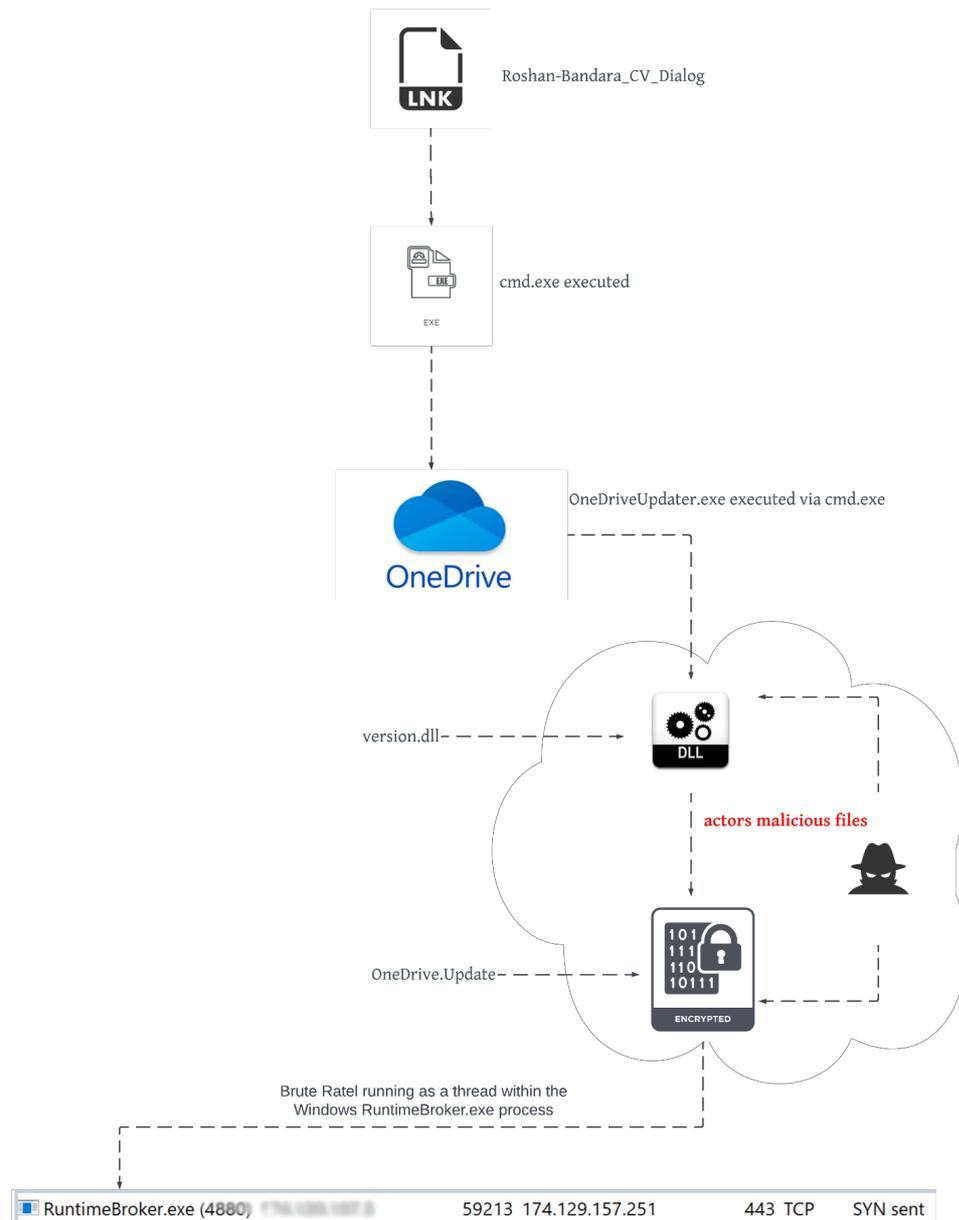
Figure 8. Execution flow when double-clicking Roshan-Bandara\_CV\_Dialog
