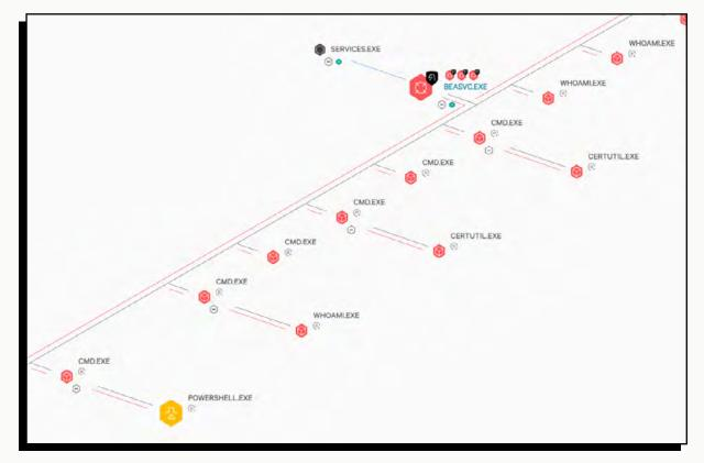
Falcon process tree showing a portion of an intrusion that exploited the WebLogic Server (beasvc.exe) process, which included several remote file copy and discovery commands.
