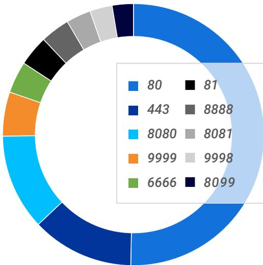
Figure 4 - Top 10 ports used for serving Beacon payloads
