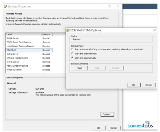
ESXi management tools can enable or disable the ESXi Shell either from within the tool, or locally on the console connected to the server. The shell defaults to "Stopped."
