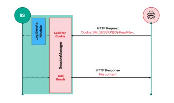
Figure 1. Malicious IIS module processing requests
