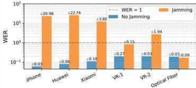
Fig. 14: WERs of sound captured by microphones and the optical fiber under ultrasonic jamming.
