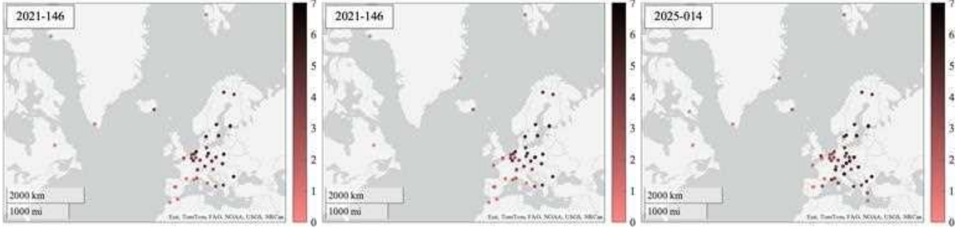
Figure 7: Detection statistic heat maps, in dB, for day 146 of year 2021 and day 014 of year 2025. GNSS receivers in the Baltic region are impacted most, which is generally representative of nearly all of the interference events.
