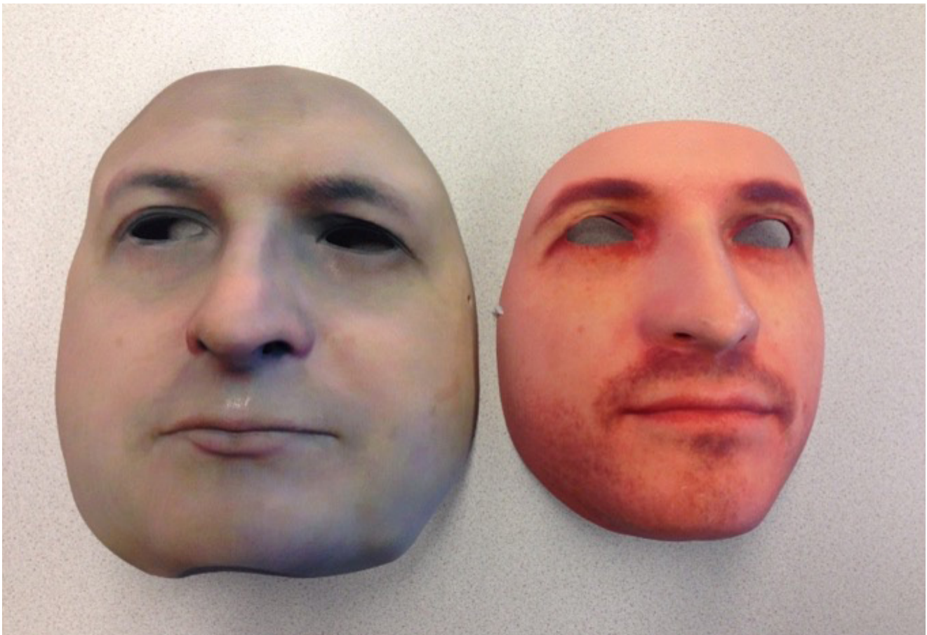
Figure 3.10: 3D rigid face masks made of resin from different manufacturers with eyes cut out. Exact 3D face shape (left) and rough approximation of the 3D shape (right) 62 .
