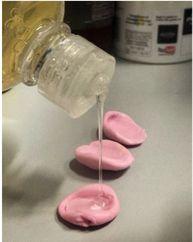
Figure 3.2: Moulding and casting method for the consensual creation of a fingerprint spoof 29 .
