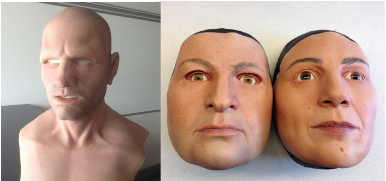
Figure 3.11: 3D flexible masks made of silicone. From left to right: a generic full-head mask and two customised half-face masks 65 .
