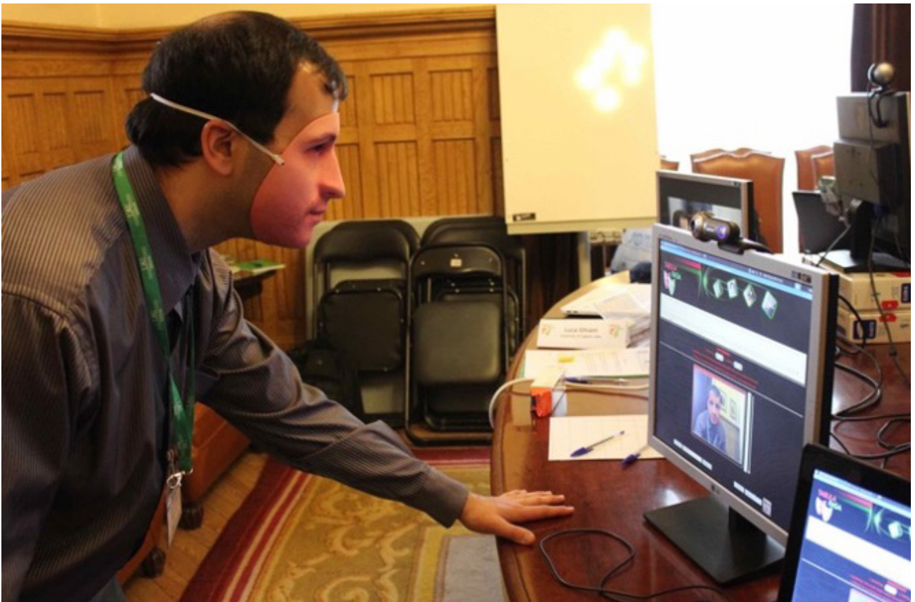
Figure 3.8: A face PA performed with a 3D rigid mask made of resin 60 .
